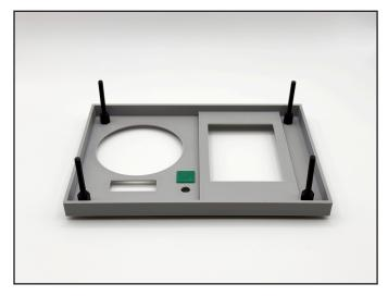
Insert the four [8] M3 (30mm) Steel Hex Screws through the [28] Top Case from the top side. Then, screw on four [5] M3 (6mm) Nylon Hex Double-Pass Spacers to hold the screws in place. Finally, insert the [27] Button into its designated opening on the [28] Top Case, ensuring it is properly seated.
