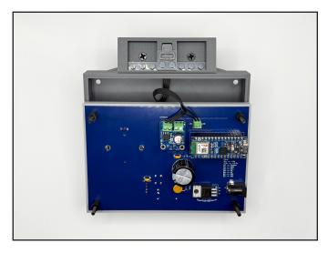
Carefully align the [1] Interface C PCB over the four exposed screws, ensuring that the LED and OLED screen are properly centered within their corresponding cutouts on the [28] Top Case. Once aligned, secure the PCB in place by fastening four [6] M3 (10mm) Nylon Hex Double-Pass Spacers onto the screws.
