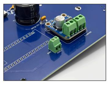
Step 13 Solder the [3] 2-pin Screw Terminal Block Connector onto the PCB. Ensure the wire holes face the direction labeled "Cable" on the PCB.
